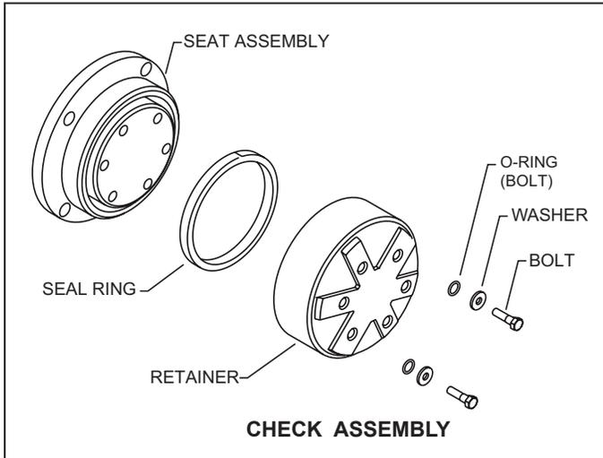
All Model 450 Double Check Valve Backflow Preventers must be inspected and maintained by licensed personnel at least once a year or more frequently as specified by local codes. Replacement of worn or damaged parts must only be made with genuine "ZURN WILKINS" parts.
