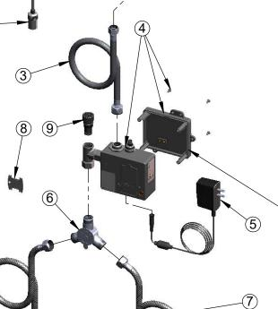
A Maximum of (8) ChekPoint Faucets can be Hardwire Connected and Powered by EC-HARDWIRE ChekPoint Hardwire AC Transformer. (Sold Separately)
