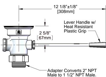
Remove Adapter When 2" NPT Male Thread is Needed.
