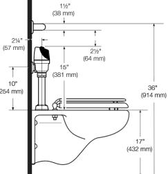
WHEN INSTALLING IN A HANDICAP STALL: Per the ADA Guildlines (section 604.9.4)
