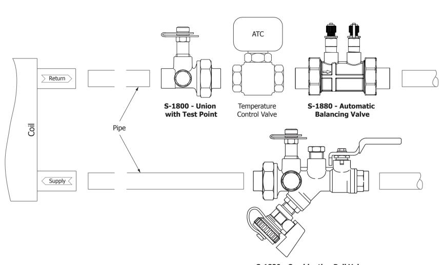
S-1820 - Combination Ball Valve with Strainer, Drain and Test Point
