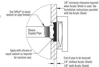
**CAUTION** Consult with supplier of acrylic, fiberglass and other non-heat resistant enclosures for recommended steamhead location. Use Acrylic Shield PN 103938 / 103938SQ. See instructions provided with steam shield. (An acrylic shield is not available for the iSteam steamhead.)
