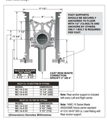
**Note:** 8" tapered thread ABS nipple shipped standard with MC-14 Series carriers. The universal faceplate assembly accepts all nipple variations, rolling thread (-OR), cast iron (-CI) and tapered thread ABS with adjustable horn (-AH).
