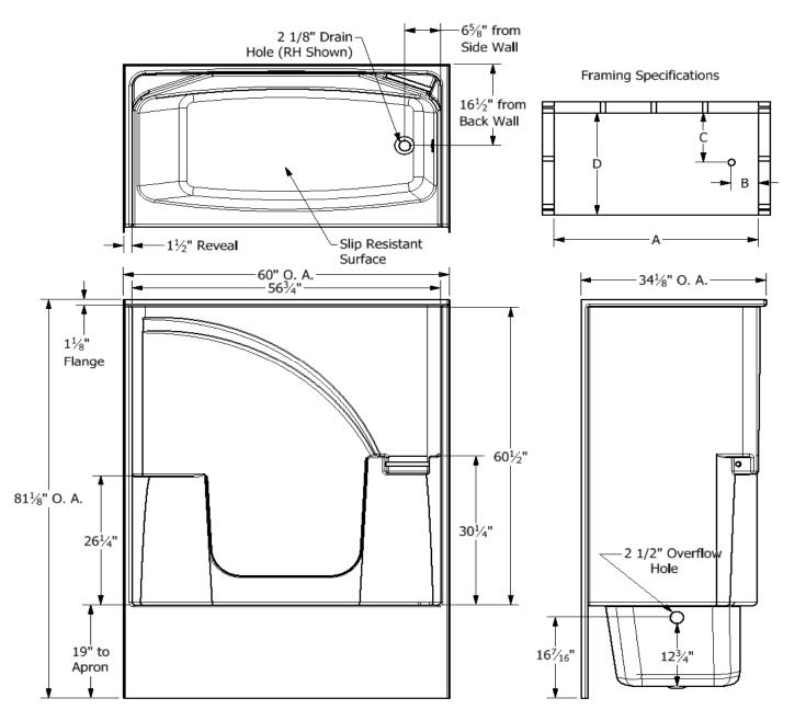
This product is tested by ICC-ES and is certified to conform to the requirements of CSA B45.5/IAMPO Z124 Manufactured by Front Line
