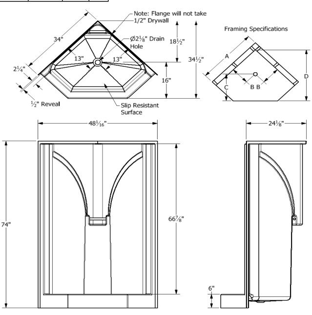
This product is tested by ICC-ES and is certified to conform to the requirements of CSA B45.5/IAMPO Z124 standard.
