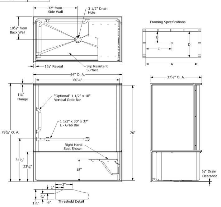
This product is tested by ICC-ES and is certified to conform to the requirements of CSA B45.5/IAMPO Z124
