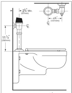
**Note:** Min. roughing height  $10\frac{1}{2}$  centerline of supply to top of fixture.
