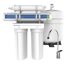
The Pentair GR0-2550 system includes the high recovery GR0-50 encapsulated membrane. The system includes a 5 micron sediment and carbon block prefilter that reduces sediment and odor and improves taste.
